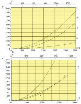
A: Pressure drop, Pa B: Airflow, m3/h C: Airflow cfm D: Pressure drop, in w.g. Top diagram: 1 = Top connection angled, Ø 200 mm 2 = End connection 3 = Exhaust rail, per metre Bottom diagram 1 = Extraction unit LL, hose 4 m, Ø130 mm 2 = Extraction unit LL, hose 4 m, Ø160 mm 3 = Extraction unit HL, hose 2 m, Ø160 mm Airflow recommendations: Heavy vehicles: 1000 - 1200 m3/h Car / SUV: 400 - 600 m3/h
